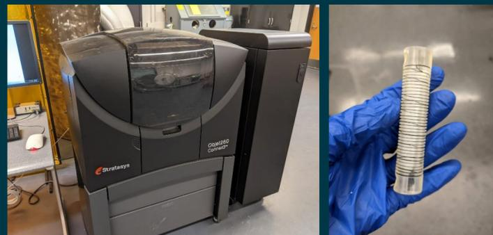
Polyjet 3D printing technology has the capability to print parts with gradient hardness. This capability is very promising in soft robot manufacturing, granting more possibilities in the robot functionalities.
